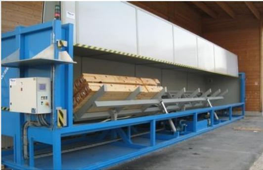
A fork lift places the load into place, the door is closed and the load is then tilted at 45°.
