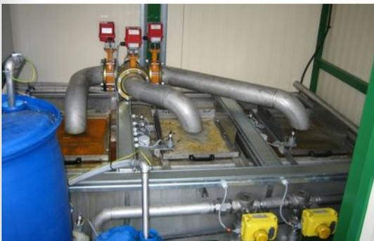
Automatic replacement of reserve solution at the end of each cycle with volumetric dosing.
